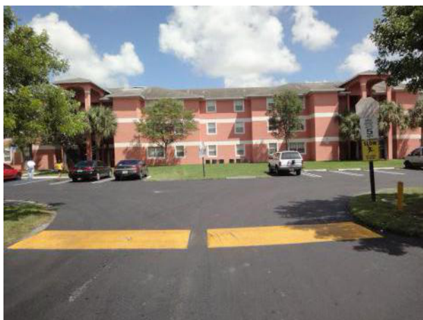
Examples of well-placed and marked speed humps for speed control. The parking lot is under natural surveillance from the windows of the adjacent apartment building units.
